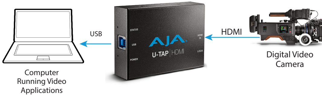
Figure 5. Typical U-TAP-HDMI Laptop System Connections
